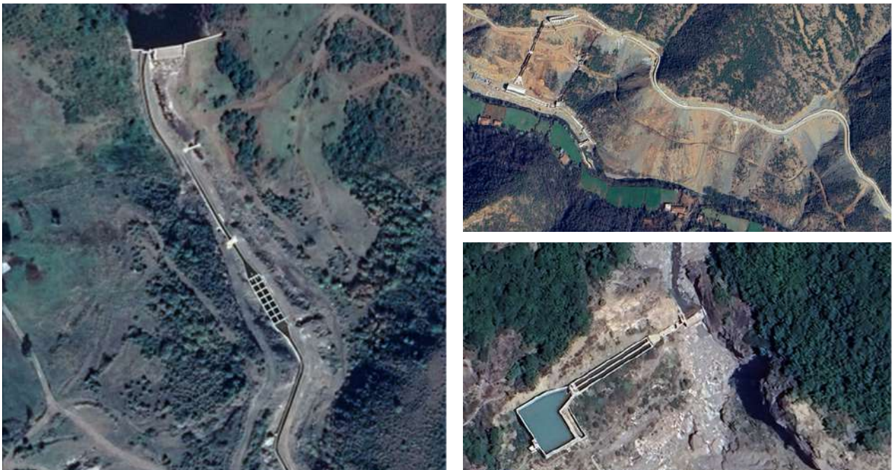
Figure 39: LEFT: Many tributaries in the eastern Drin catchment are impacted by hydropower water abstraction (nearly 100% of the water), Albania. UPPER RIGHT: Construction site on the Shkumbin tributary in Albania. The pipes carrying abstracted river water are often built into steep mountain slopes, leading to long-term erosion. LOWER RIGHT: Total water abstraction in June 2025 (HPP Lubonje (0.1-1 MW), upper Osum tributary, Albania. © GE 2025
