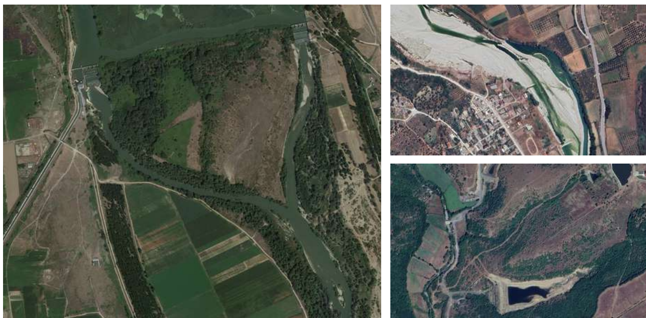
Figure 45: LEFT: Axios GR (left and right-side water abstraction upstream of lower course and delta). © GE 2025. UPPER RIGHT: Shushica (temporal excavation after each flood, diversion of water to the top left corner). © GE 2025. LOWER RIGHT: Many small reservoirs not serving only for drinking water have been built and will be built, altering many catchments of all sizes AL. © GE 2025
